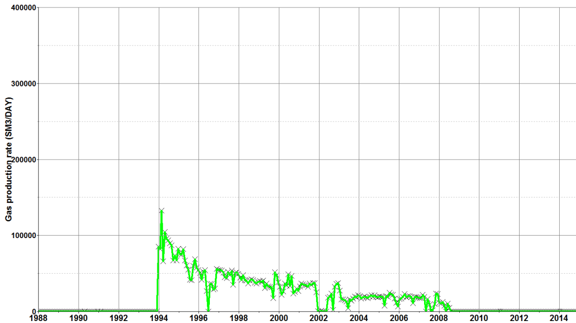
Figure 15-33 HRL-08 HM, gas production rate (green line = history match, black line = original history match, red line = Franeker sensitivity, black crosses = historical data)
